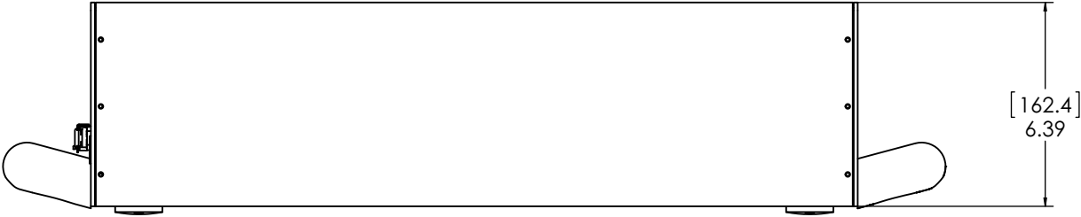
Figure 4-2. Vitara Laser Head Dimensions (Side View)
