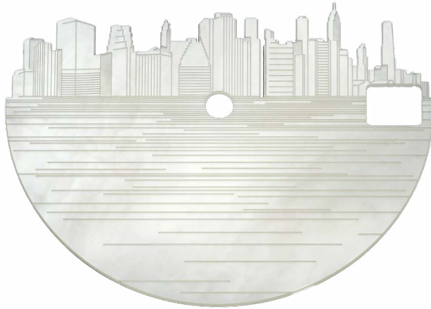
This city skyline was laser cut by TechnoCut in mother of pearl which is often used for decoration of premium brand watch faces. No post-processing was required. Image courtesy of TechnoCut.
