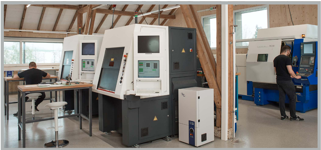
TechnoCut currently uses four MPS machines from Coherent, all equipped with femtosecond lasers. Image courtesy of TechnoCut.
