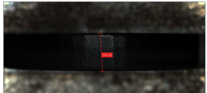
Inner edge of cut holes with 100 W, 10.2 μm wavelength CO 2 laser
